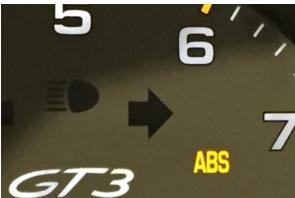
ABS is the oldest technology (on Porsches since 1985) and fortunately one that the driver and instructor can feel and (usually) hear. It is also easy to use as a learning tool. If ABS has been activated on a dry track, the driver has just driven over the limit and it's time to brake earlier. For those looking for the last tenth, remember that peak braking force occurs just <u>before</u> ABS kicks in.
