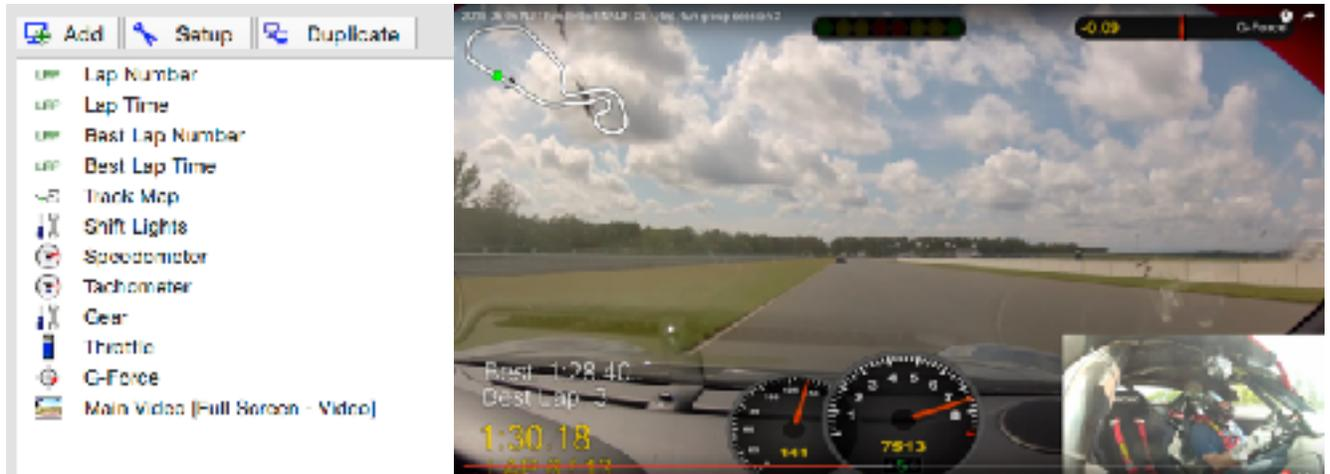
**Vbox CircuitTools** is another terrific piece of software that combines Video with “squiggly line” data analysis in a single integrated view. So far it only works with their own Vbox video loggers but it can read just about any data logger’s lap data. CircuitTools has well-executed user experience combining synchronized video with lap segments, split times, color coded track map and “squiggly line” G-Force data graphics all on a single four quadrant screen.
