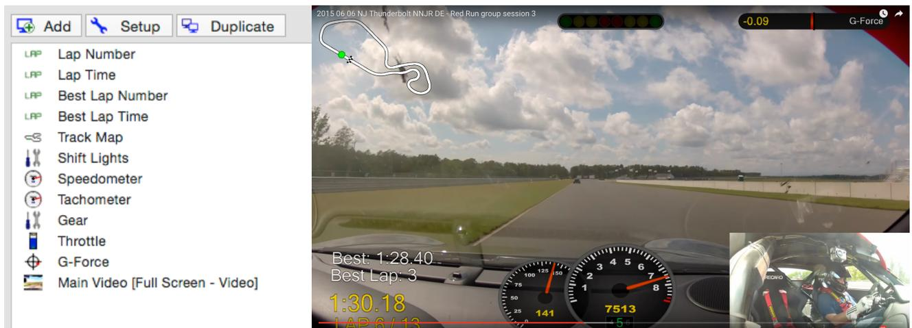
**Vbox CircuitTools** is another terrific piece of software that combines Video with “squiggly line” data analysis in a single integrated view. So far it only works with their own Vbox video loggers but it can read just about any data logger’s lap data. CircuitTools has a well-executed user experience combining synchronized video with lap segments, split times, color coded track map and “squiggly line” G-Force data graphics all on a single four quadrant screen.
