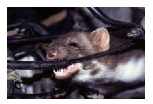
The rodent had quite a penthouse pad behind the right taillight assembly. Ninety percent of the foam insulation that is usually above the engine, was now finely mulched into a big nest with plenty of dog food bits, broken wires (11 different colors), and topped off with extra urine. The clean up became a near hazmat infectious task from hell.
