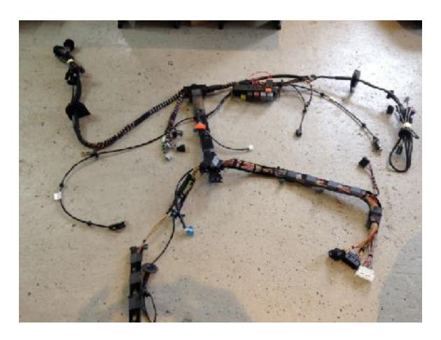
Just for reference, the thick central part goes under the e-brake handle and almost all the interior had to come out.
