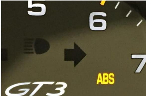
ABS is the oldest technology (on Porsches since 1985) and fortunately one that the driver and instructor can feel and (usually) hear. It is also easy to use as a learning tool. If ABS has been activated on a dry track, the driver has just driven over the limit and it's time to brake earlier. For those looking for the last tenth, remember that peak braking force occurs just before ABS kicks in.
